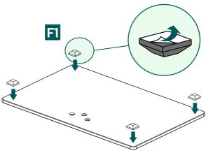
• Attach the self-adhesive rubber feet [F1] to the corners of the base plate as shown above.
