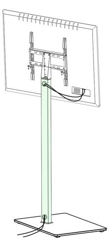
• Use the openings on the mounting pillar for cable management.
