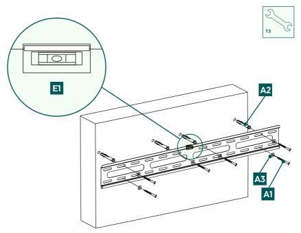
• Attach the wall bracket to the wall as shown above using the enclosed mounting material ([A2] plug, [A3] M8 washer, [A1] 8x60 mm screw and the [E1] spirit level).
